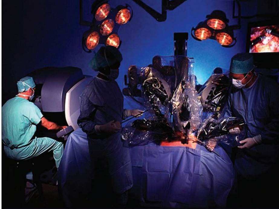
A surgeon controls the robotic instruments with hand devices and foot pedals as he sits at the console of the da Vinci® Surgical System.
